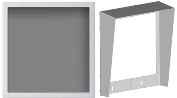
Part No. 9135362E Flush mounting box with 2-module roof Roof dimensions (WxHxD) : 229 x 240 x 41 mm Hole (WxHxD): 210 x 220 x 50mm +- 5mm
